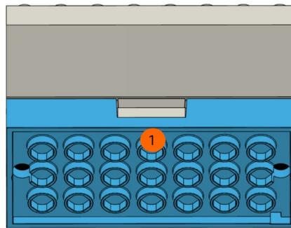
You can select from 3 power modes using the supplied magnetic cable tie (or any magnet). Hold it beneath the status indicator (marked (1) in the figure above) until the status indicator flashes.
