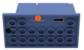
You can select from 3 power modes using the supplied magnetic cable tie (or any magnet). Hold it beneath the status indicator (marked (1) in the figure above) until the status indicator flashes.
