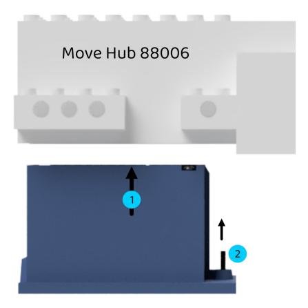
Start removing the original battery cradle by removing the screw on the bottom of the hub.
